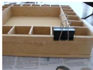
**Step Three:** Use Wood Glue to stick the plain base strip on the bottom and clamp in place until it dries. This base strip helps the Advent Calendar to sit straight and not fall forward.
