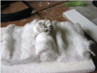
**Step Eight:** Pack the ring carefully with fibre cloth so it is sitting upright. Be careful not to pack it too tightly otherwise it will crack when it shrinks as its firing. Fire for 5 minutes at 800oC.
