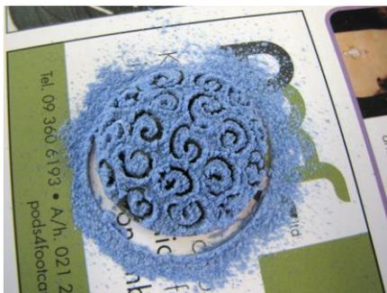
11. Carefully lift the disc on to the trivet and place in to the kiln. Fire.
