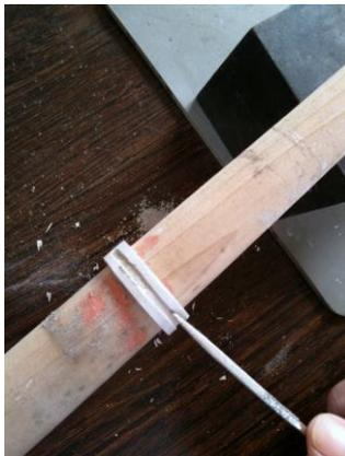
Step Two: Make a pencil line around the ring, where you want the inlay to be. Using a square edged file, slowly work your way around the pencil line to make the inlay. The filed line can be made with a standard file and then carved out with a craft knife but you must end up with a carved out square shape with no rounding at the bottom.
