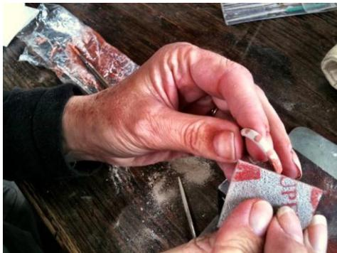
Step Seven: Sand evenly using the red coloured sponge sandpaper. Keep going until you reach the silver and your copper pattern comes through. Check for areas where there is no copper. Even little pin sized holes need to be filled, dried and resanded.
